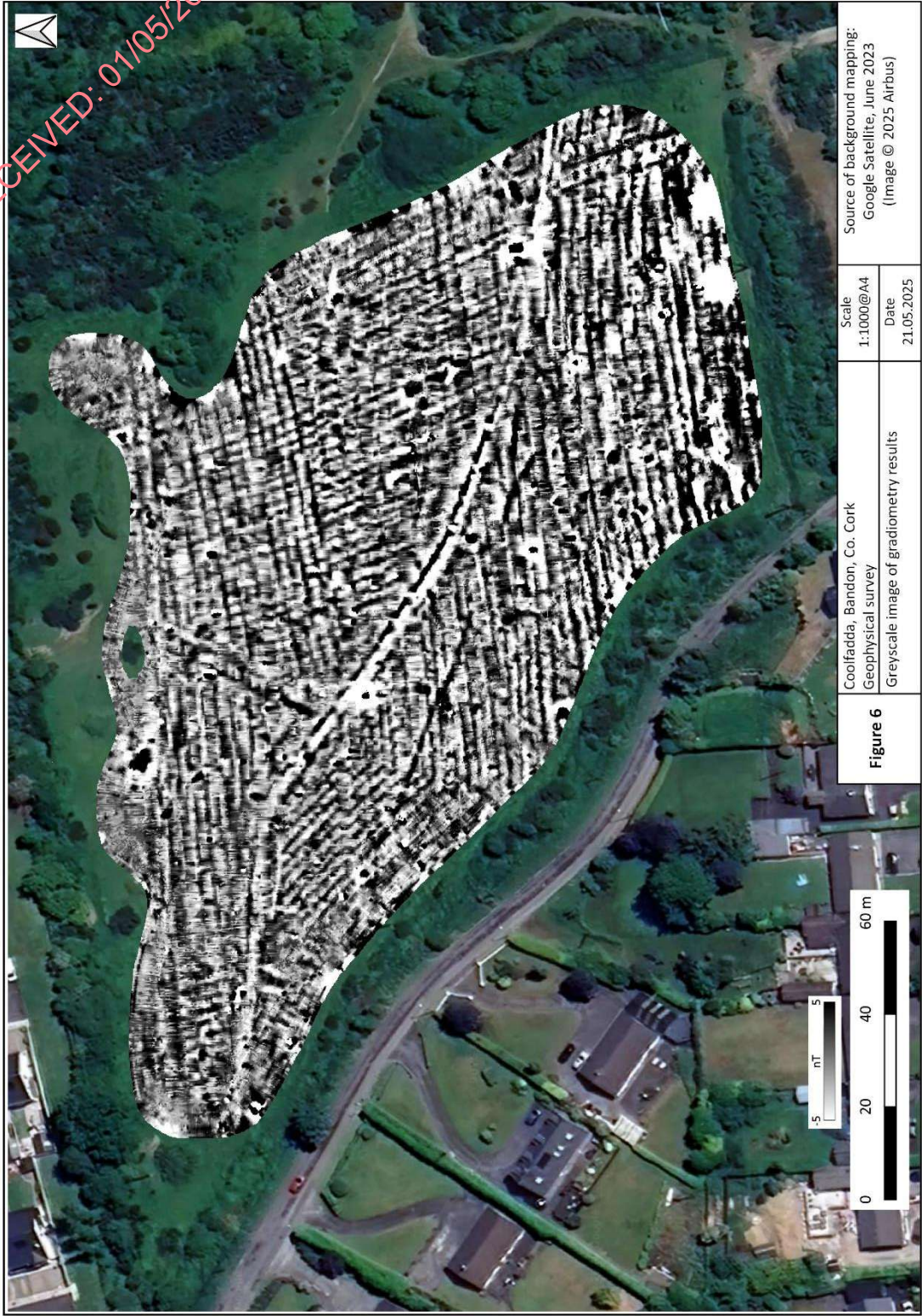
Figure 6. Greyscale image of gradiometry results.
